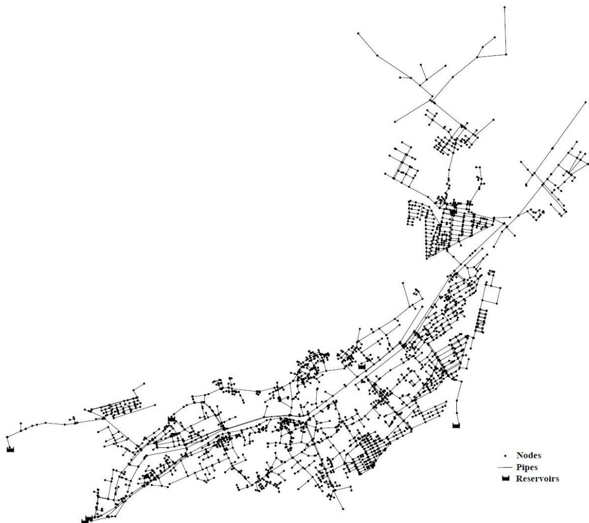
Fig. 2- Taft water distribution network model
