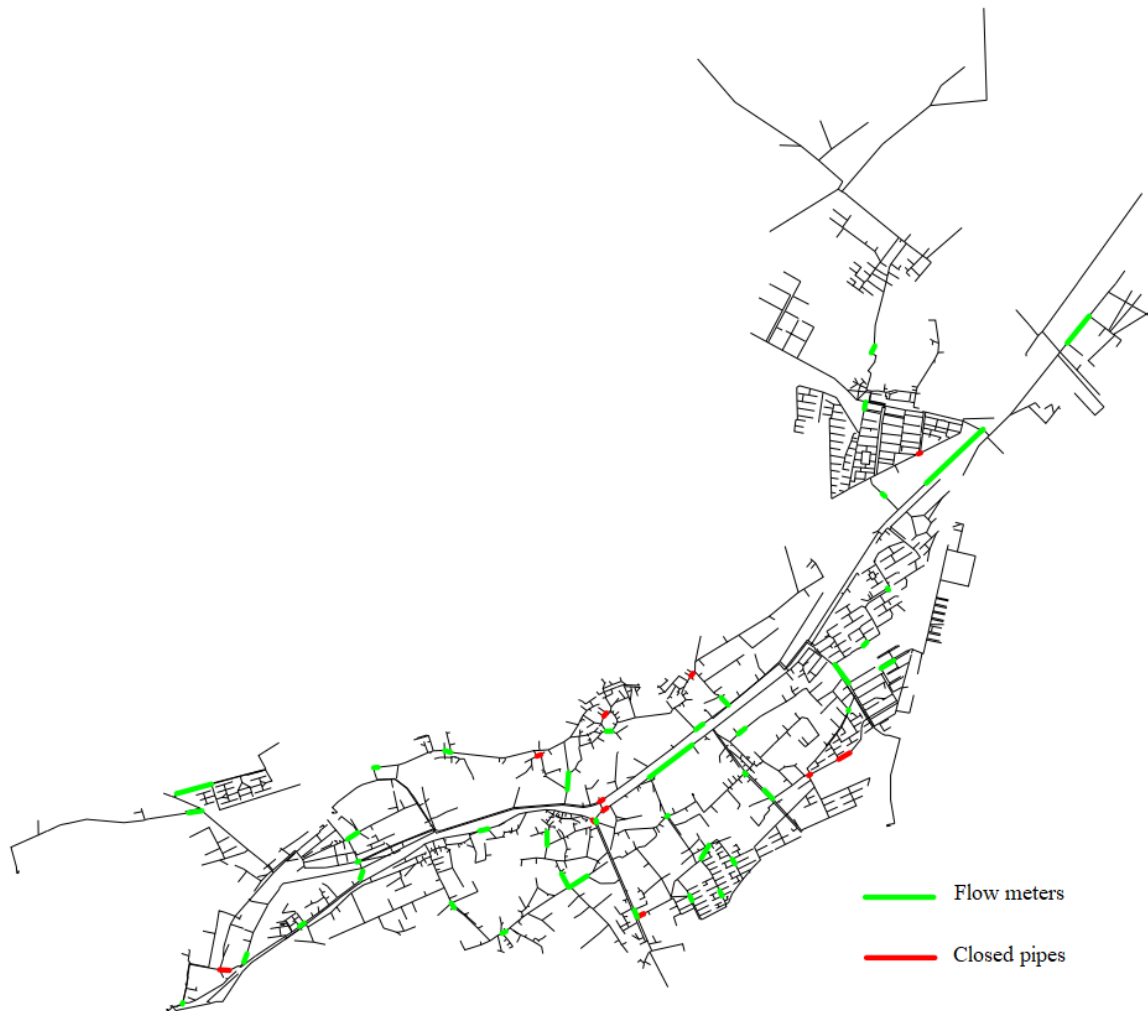
Fig. 4- Boundary pipes optimization results
