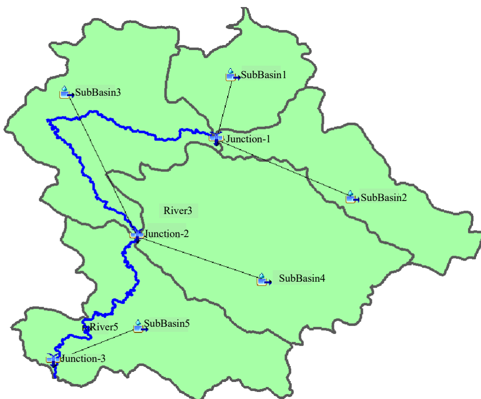
Fig. 2- Schematic of the Poldokhtar basin in the HEC-HMS hydrological model in this study
